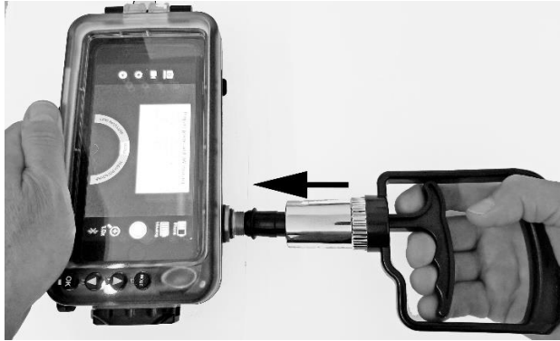
Hand pump pressed against vacuum check port
