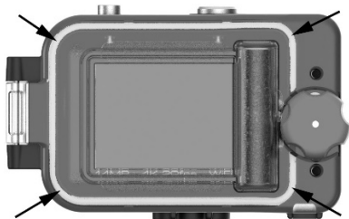
Check O-ring seal is good
