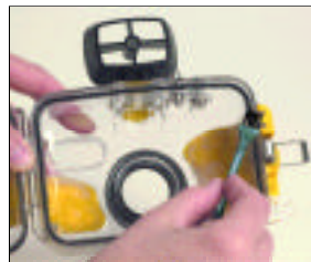
Clean O-Rings w/Brush Insert Desiccant Do not grease O-Ring
