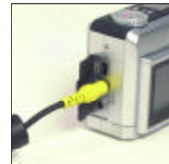
Connect Video Cable to Video-In at back of TV set and the other end to the camera
