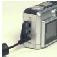
Plug Power Cable into camera jack (DC/6 volt)
