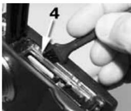
4) Use the cleaning brush provided to remove any sand or debris from the O-ring groove, waterproof door and sealing area.
