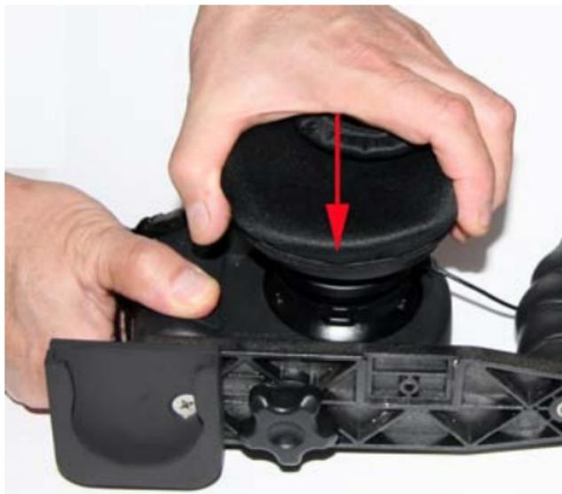
Push lens onto lens port of any SeaLife “DC”-series underwater camera. Lens can be attached on land or underwater. When entering the water, make sure to remove air bubbles trapped under the lens - There should be water between the lens and the camera.
