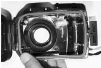
Step 3: Carefully close housing to firmly seat O-ring and open housing again to inspect that O-ring is completely seated into groove. Do NOT grease the O-ring.
