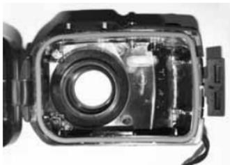
Step 1: Lay the O-ring over the O-ring groove making sure the O-ring is not twisted. Orient the O-ring with the more rounded corners on the hinge side of the housing.
